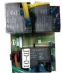
Contactor (3 phase relay)
