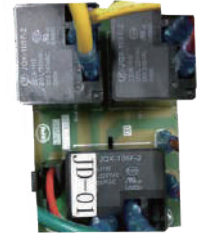
Contactor (3 phase relay)
